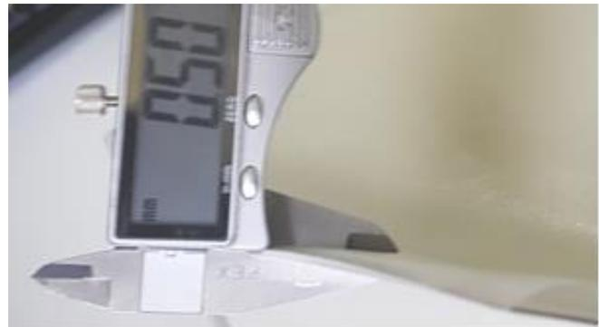
Fig. 3. Thickness measurement of paper in a sleeve, which determines the distance between each pair of tags.
