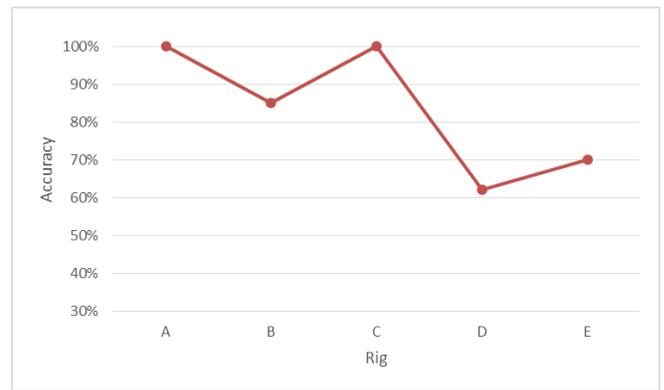
Fig. 8. Results of tag scanning (open environment – dynamic reading).
