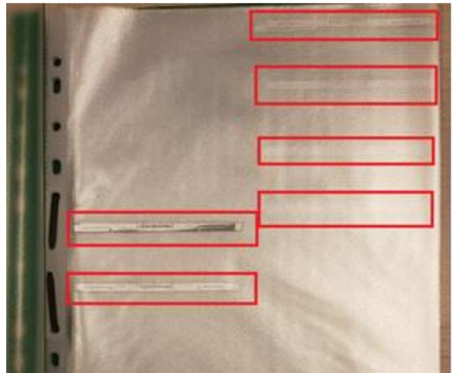
Fig. 1. Test rig B with marked stacks of tags, each with 2 tags – photo taken before inserting paper in the sleeves.
